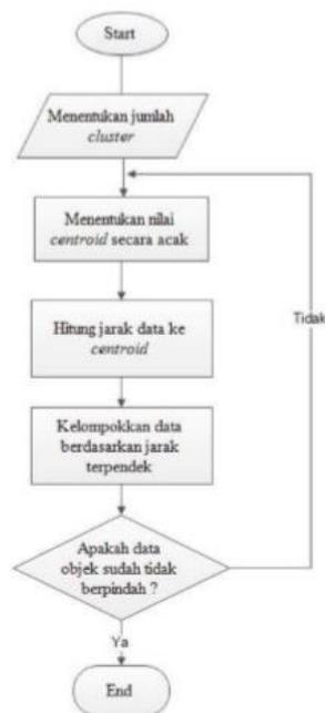
**Gambar 2.5 Flowchart Algoritma K-Means**
