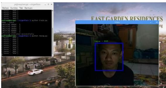
**Figure 16.** Testing facial recognition accuracy with 5 data training
