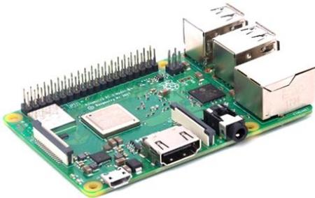
Figure 1. Raspberry Pi 3 Model B
