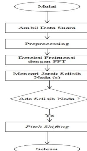
Gambar 4. Diagram Alur Pencocokkan Nada
