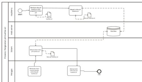
Picture 3 BPMN pH Monitoring water quality Built
