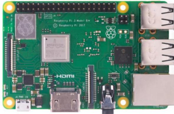
**Gambar 2.2** Raspberry Pi 3 Model B+ [21]
