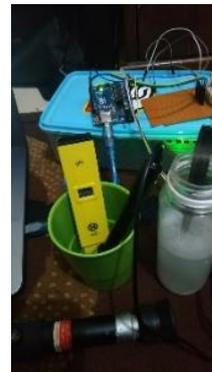
**Figure 7** Testing the pH sensor SEN0161
