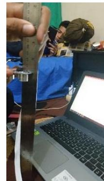
**Figure 10** Testing of Ultrasonic Sensors HC-SR04
